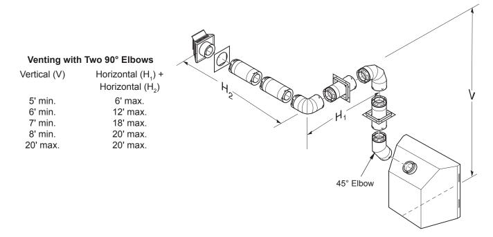
Figure 18 - Horizontal Termination Configuration for Venting Using Two 90° Elbows with Termination at 90° with Fireplace
